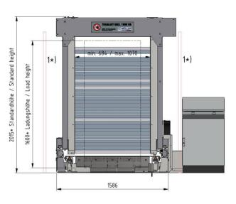
\*1) In automatic operation, separating devices and contactless protection systems (light barriers) must be provided for personal protection
