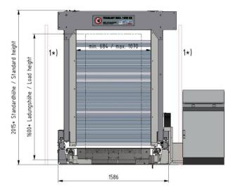
\*1) In automatic operation, separating devices and contactless protection systems (light barriers) must be provided for personal protection
